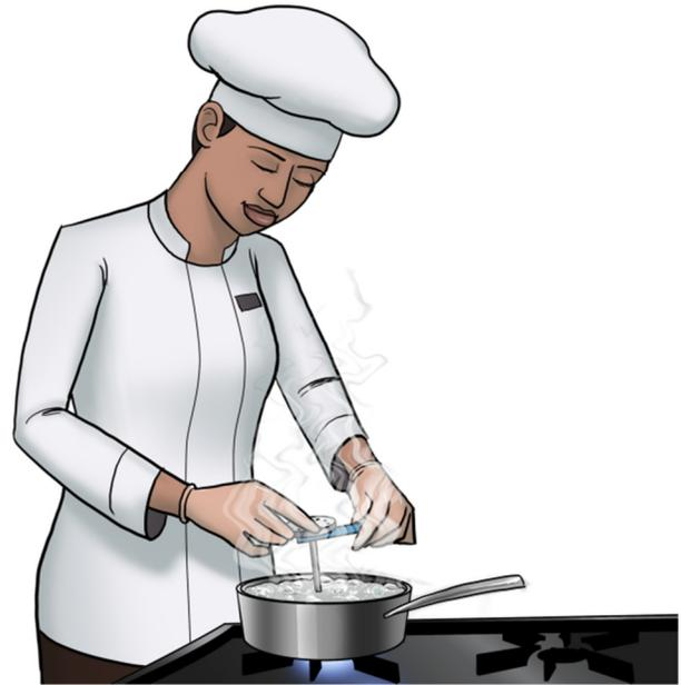
methods for calibrating thermometers, but the principle behind calibration is always the same: to calibrate a thermometer, put it in a substance with a known temperature and adjust the thermometer's calibration mechanism as necessary to arrive at the known correct reading.
